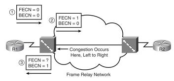
FECN and BECN are bits in the Frame Relay header. At any point—either in a router or inside the Frame Relay cloud—a device can set the FECN bit, meaning that this frame itself has experienced congestion. In other words, there is congestion in the forward direction of that frame. In Figure F-2, at Step 1, the router sends a frame, with FECN=0. The Frame Relay switch notices congestion, and sets FECN=1 at Step 2.
