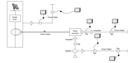
Figure 1-7 Hybrid Fiber Coax Cable (HFC) Network
