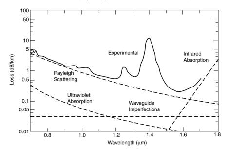
Figure 1-4 Attenuation Curve in a Fiber (Reprinted from IEEE Electronics Letters, 1979)
