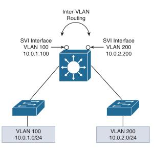
Figure 1-5 Inter-VLAN Routing via SVI
