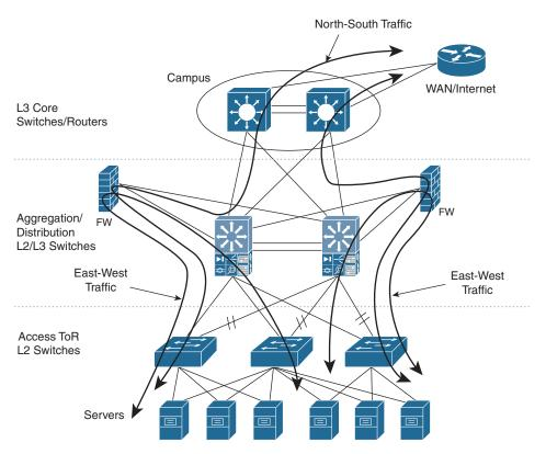
Figure 1-9 Firewall Overload
