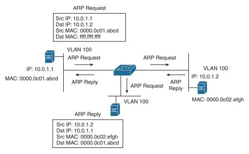
Figure 1-7 ARP Flooding
