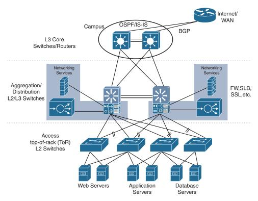
Figure 1-1 Networking View of Three-Tier Data Center
