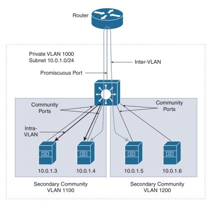
Figure 1-6 Primary and Secondary VLANs
