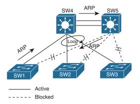
Figure 1-8 Loop Prevention Via Spanning Tree
