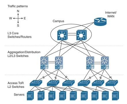
Figure 1-3 The Challenge of Scaling Three-Tier Designs
