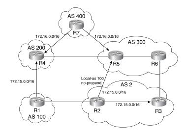
The next step is to migrate R1 to the new AS. Local AS is configured on R1 on the session with R4. AS\_PATH prepending is now removed on R1. The LOCAL\_PREF is modified to prefer the path via R4. The reason that LOCAL\_PREF is used instead of WEIGHT is that R2 would also prefer the path via R1 for 172.16.0.0/16 if the link between R2 and R5 failed. The new BGP configurations on R1 and R2 are shown in Examples 4-50 and 4-51, respectively.
