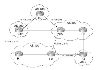
For the purposes of this case study, the last octet of an IP address indicates the router number. Basic BGP configurations for R1 and R2 are shown in Examples 4-40 and 4-41, respectively.
