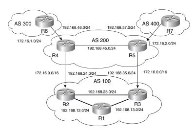
Figure 4-4 Example of Conditional Injection
