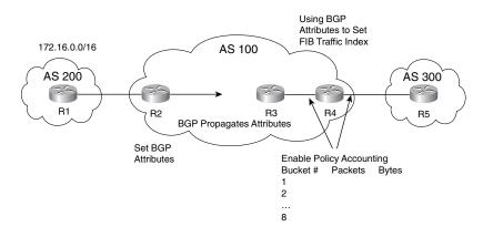
**NOTE** Remember that changes to the FIB/RIB tables are updated when the IP RIB is cleared using **clear ip route** \*, the BGP session is reset, or a router is reloaded. All these actions can be disruptive to the traffic.
