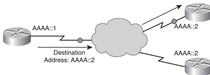
**Figure 7-3 IPv6 Anycast Example**
