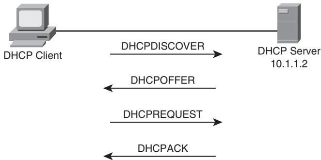
**Figure 10-1 DHCP Messages Exchanged Between a DHCP Client and a DHCP Server**
