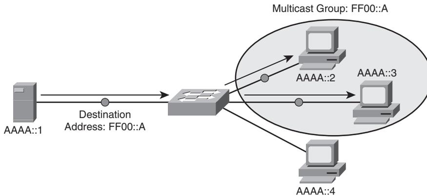
**Figure 7-2 IPv6 Multicast Example**
