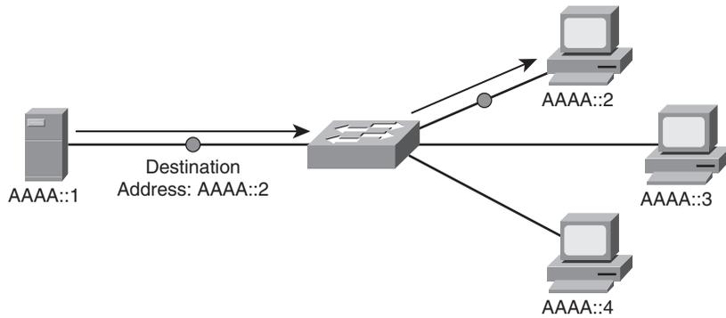
**Figure 7-1 IPv6 Unicast Example**
