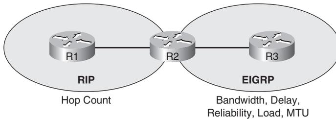
**Figure 5-2 Differing Metric Parameters Between Routing Protocols**
