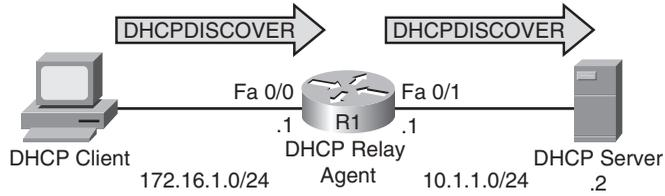
Figure 10-3 A DHCPDISCOVER Message Forwarded by a Router
