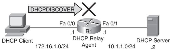
**Figure 10-2 Router Blocking Broadcast Traffic**
