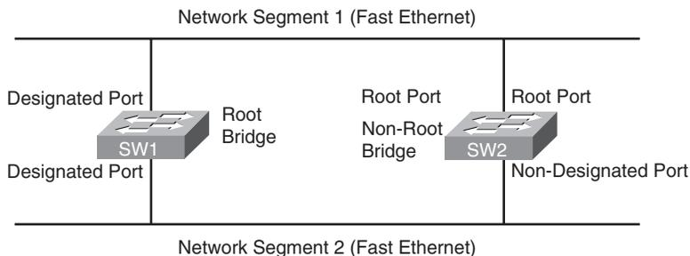
**Figure 1-2 STP Port Assignments**
