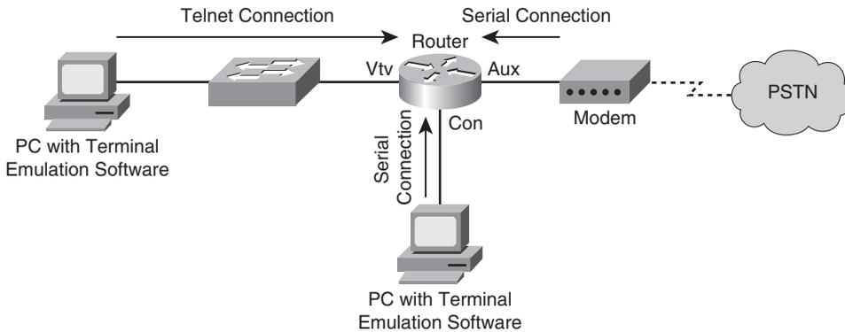
**Figure 9-1 Router Password Protection**
