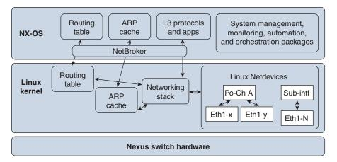
Figure 7-5 NetBroker—Synchronize NX-OS and the Linux Kernel
