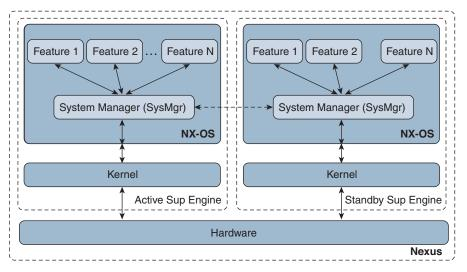
Figure 7-2 NX-OS Fault Detection and Recovery
