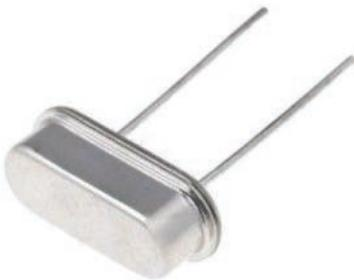
**Figure 5-1** 16-MHz Crystal Oscillator
