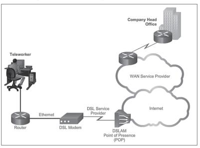
The topology in Figure 2-23 displays a sample DSL WAN connection.
