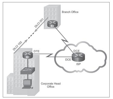
Figure 2-18 Sample Frame Relay Topology
