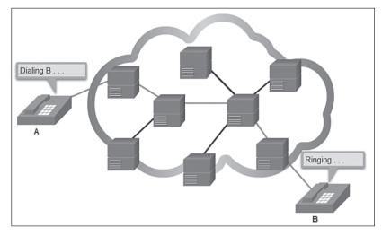
Figure 2-9 Circuit-Switched Connection
