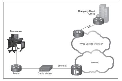
The topology in Figure 2-24 displays a sample cable WAN connection.
