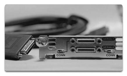
Figure 3-14 Smart Serial Connector
