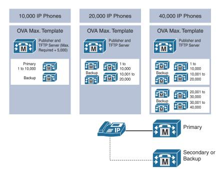
Figure 2-11 1:1 Redundancy Design
