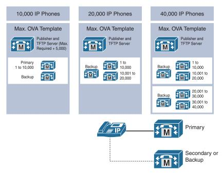
Figure 2-12 2:1 Redundancy Design
