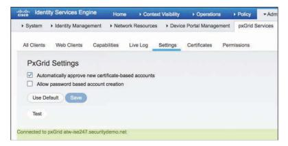
**Figure 6-21** Enabling Automatic Approval of Certificate-Based Accounts in pxGrid Settings
