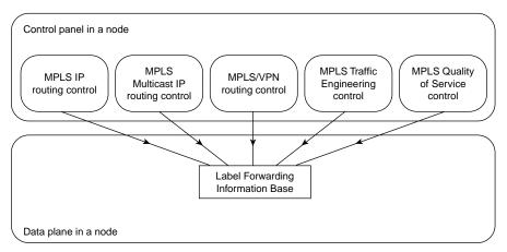
Every MPLS application has the same set of components as the IP routing application:
