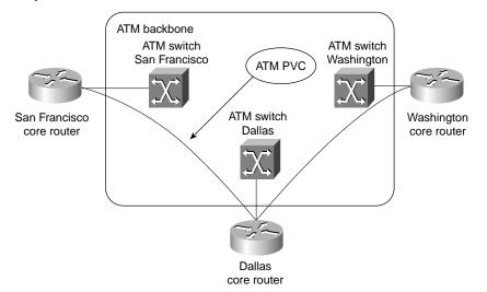
Figure 1-1 Sample IP Network Based on ATM Core
