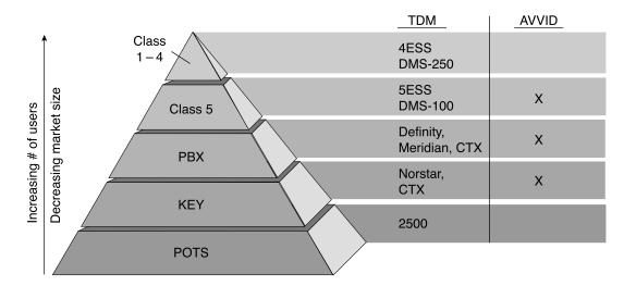
Figure 1-7 Cisco AVVID IP Telephony Scalability
