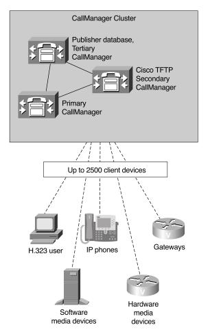
The second deployment model has the advantage of eliminating the risk that database activity on the Publisher database degrades performance of CallManager if the primary CallManager is unavailable. Furthermore, both deployment models permit the use of the locations feature of CallManager as an admissions control mechanism. (Admissions
