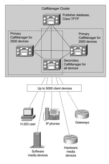
Figure 1-14 Deployment Model for 2500 to 5000 Users
