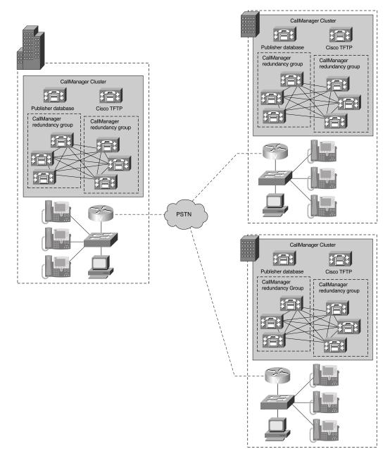
Figure 1-18 Multiple-Site Model with Independent Call Processing
