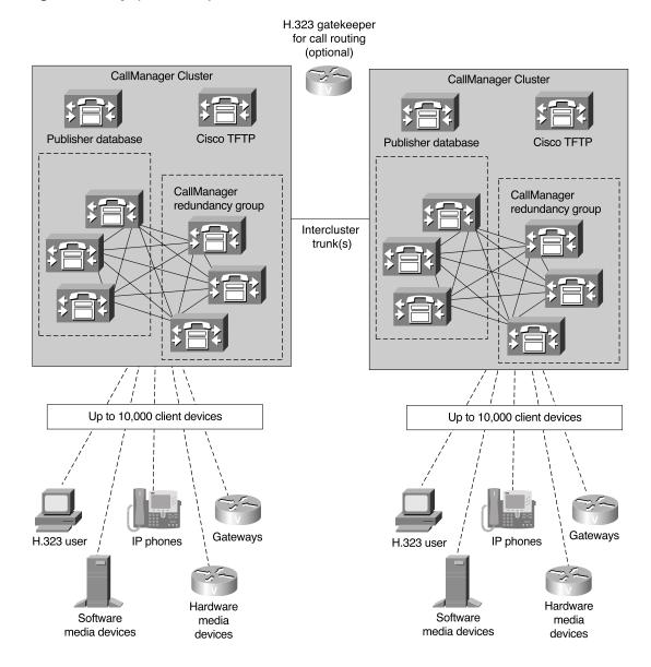
Figure 1-16 Deployment Model for More than 10,000 Users
