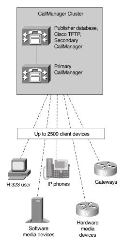
The second deployment model requires a third server. In this model, the first server houses the Publisher database and Cisco TFTP. The second server houses a primary CallManager. The third server houses a backup CallManager. Under normal operating conditions, call devices in the cluster register to the second server, but if the second server is unavailable, the third server takes over CallManager responsibilities. Figure 1-13 shows this deployment model.
