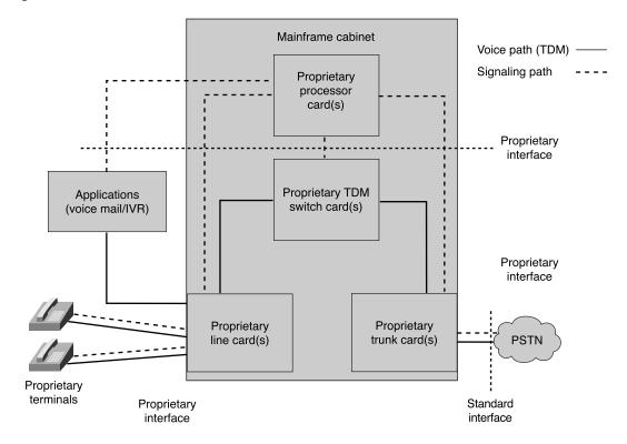
Figure 1-2 Traditional Circuit-Switched Architecture
