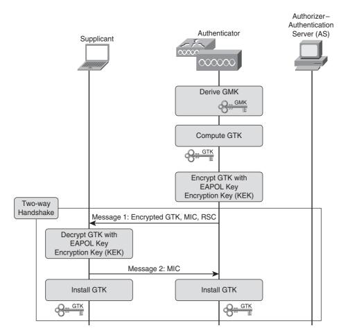
Figure 4-13 Group Transient Key Two-Way Handshake
