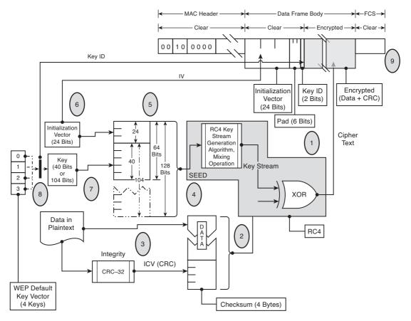
Figure 4-1 WEP Processing Model
