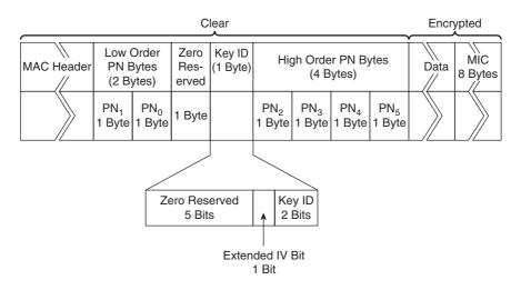
Figure 4-18 CCMP Packet Format
