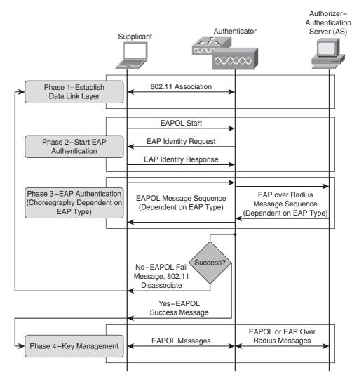
Figure 4-5 illustrates the 802.11i authentication framework.
