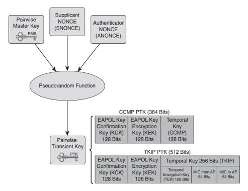
Figure 4-11 Pairwise Transient Key Generation
