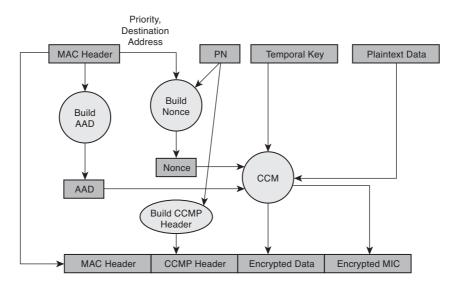
Figure 4-19 CCMP Encapsulation Process
