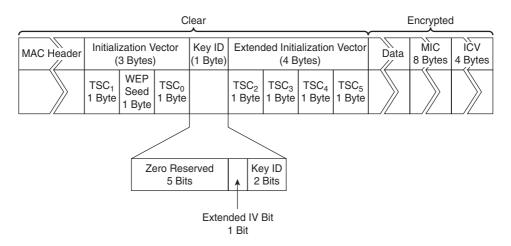
Figure 4-14 TKIP Packet Format
