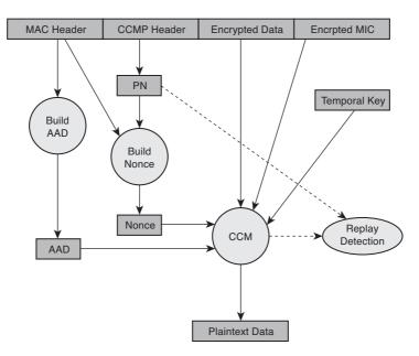
Figure 4-20 CCMP Decapsulation Process
