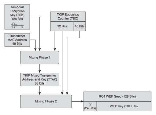
Figure 4-15 TKIP Key-Mixing Algorithm
